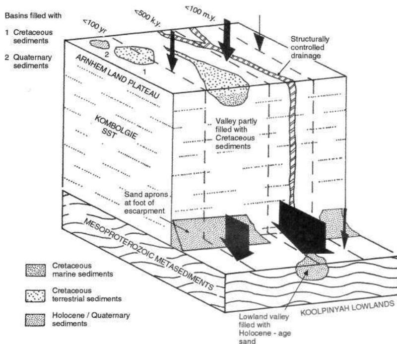
**Figure 2.** Schematic diagram of Arnhem Land plateau and Koolpinyah lowlands, showing denudation over different time scales. Width of arrow on each of the time-lines represents rate of denudation. Note angular unconformity at base of escarpment coinciding with lowland Koolpinyah surface, and fades transition from Cretaceous marine to terrestrial sediments within upland valley (after Nott and Roberts<sup>2</sup>).
