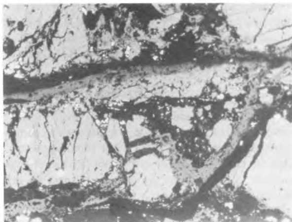
Figure 7. Two generations of uraninite grains (lighter grey), and more oxidised supergene veins and patches (darker grey). The small scattered white grains are galena. (Magnification 200X).
