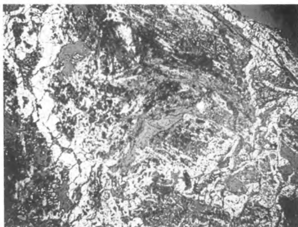
Figure 5. Remobilisation and redeposition of uraninite (white mineral). Photomicrograph shows uraninite veins (left and right) partially destroyed by dissolution of uranium which has been redeposited as scattered veinlets and shapeless masses of a new generation of uraninite (middle). (Magnification 10X).
