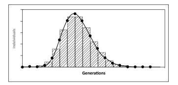
**Figure 4.** Principle of numerical integration. The x axis is divided into discrete interval widths. The height of each is the average of the y value at the beginning and end of each interval. All the areas are then summed.
